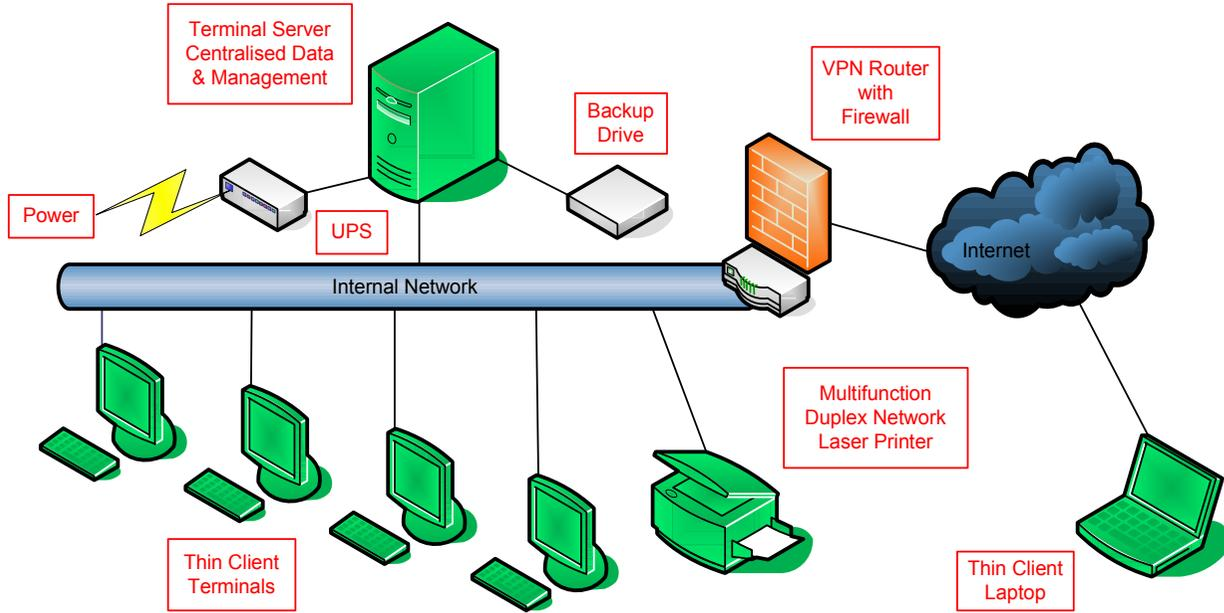
This is a comparison example between 4 Standard PCs plus a Server versus 4 Thin Client Terminals plus a Server. Thin Client Terminals have no moving parts, such as, fans, hard drives etc, therefore have an extended life over a conventional PC.
